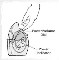
Place receiver in room in which you intend to use it. Rotate the power/volume dial to turn power on. Power indicator lights. Adjust receiver location.
